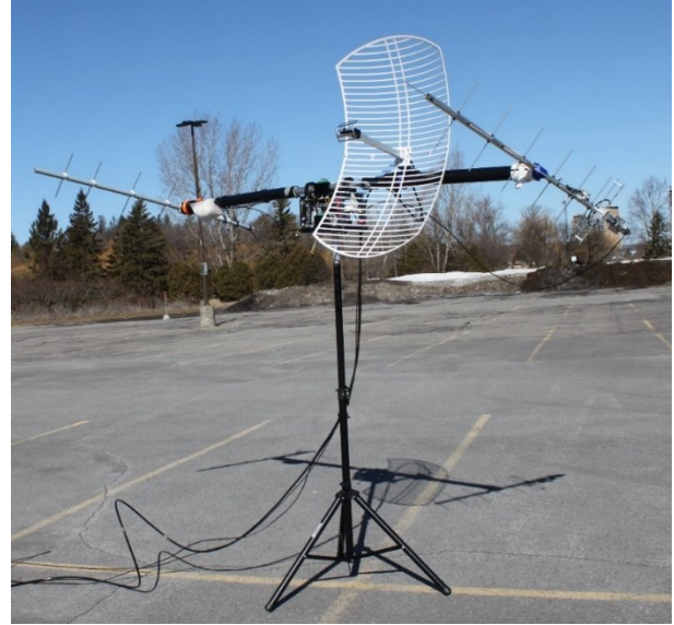
Fig. 7: Current ground station configured for UHF (TX/RX) and L-Band (RX)
