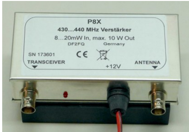
Fig. 11: P8X Power amplifier
